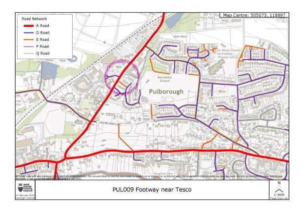
**Issue**: Pavement narrowed by street furniture and bus infrastructure near the entrance to Tesco which reduces the footway width. There has been a recorded injury accident in this area.
